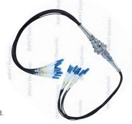
Fiber Optic Rotary Joints (FORJs) are to optical signals what electrical slip rings are to electrical signals, a means to pass signals across rotating interfaces, particularly when transmitting large amounts of data. FORJs maintain the intrinsic advantages of fiber end to end. JINPAT has been producing Fiber Optic Rotary Joints for over Twenty-five years..
